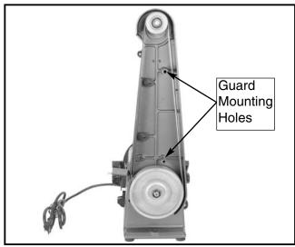
Figure 3. Outside belt guard attachment points.
